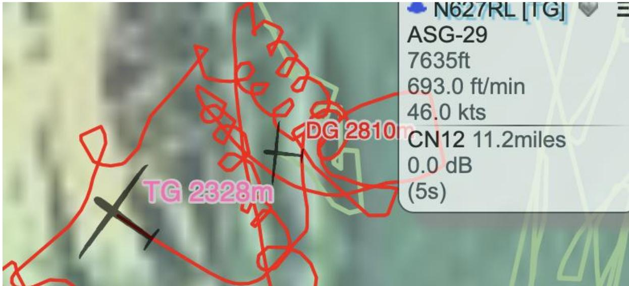
After clicking on a target, a panel opens on the right side of the screen. The last number in parenthesis tells how much time since the target was last seen. Above that is the signal strength and the receiver that last picked them up and the distance from that receiver. There is also the altitude, climb/sink rate, and forward speed.
