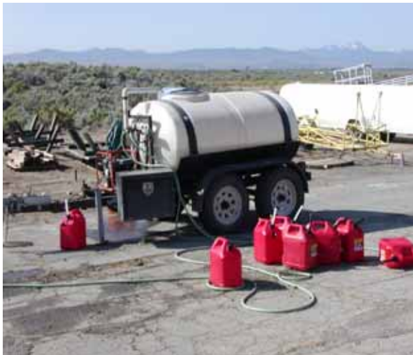
Loading water ballast was done from this custom built pumped water tank, courtesy of Rick Walters.
