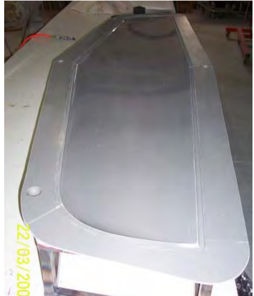
March 2005: Horizontal tail molds done
